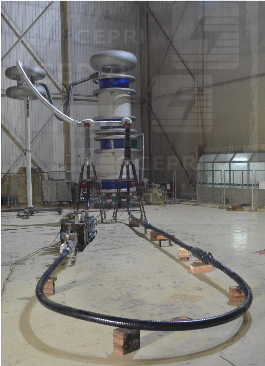
Figure C.1 The test loop of sample tested
